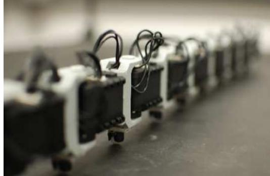
Figure 1: A planar tentacle robot with ten links.
