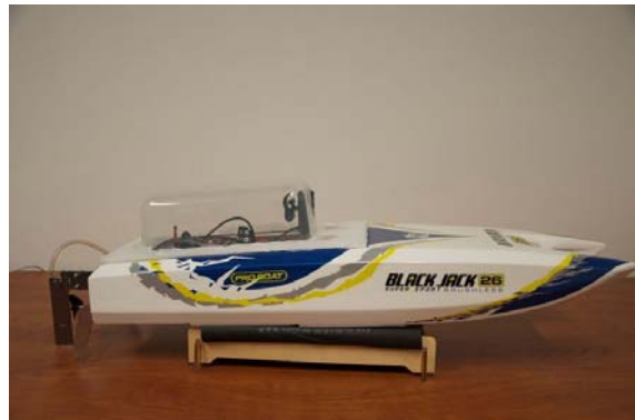
Figure 1: The “minnow”. The autonomous service vessel is constructed from a modified RC motorboat, and has been augmented with onboard electronics and sensors. An 802.11g network connection provides offboard communication.
