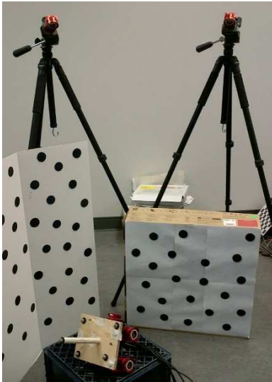
Figure 8: The camera cluster constructed for these experiments is mounted on a hand-held rig and augmented with IR reflecting markers for ground truth data collection using the motion capture system (shown on tripods in the background). The target object consists of the black dots on the white background.
