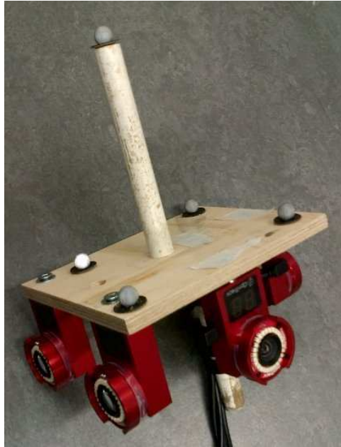
Figure 1: Multiple perspective cameras are arranged to form a camera cluster such that they cover as large an FOV as possible, even with no spatial overlap. This cluster consists of four cameras, two forward, one sideways and one backward-facing, at known positions and orientations.
